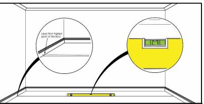
Height Measurements need to be taken from a level base. From the **highest** point of the floor at the very front of the wardrobe depth, set a level. This can be done with a long spirit level – Laser or packed length of timber. (make sure you include the thickness of the timber when measuring)
