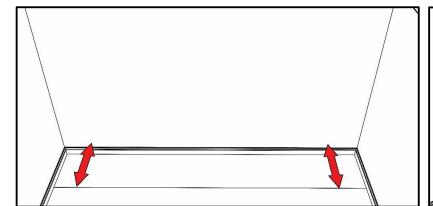
From the back wall measure the depth available. The measurement needs to be taken from the wall not the skirting board (recommended depth is 650mm or 700mm if it is a full carcass wardrobe)
